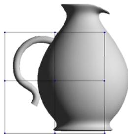
Position of undeformed lattice
