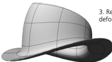
3. Result of a second deformation (Twist)
