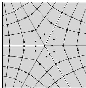
The multiknots create a discontinuity that helps align the surfaces. Continuity is maintained across the multiknot curves as if they were junctions.
