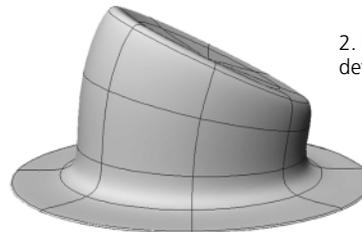
2. Result of a deformation (Bend)
