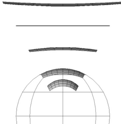
Effect of different Amplitude values on a grid shrinkwrapped to a sphere
