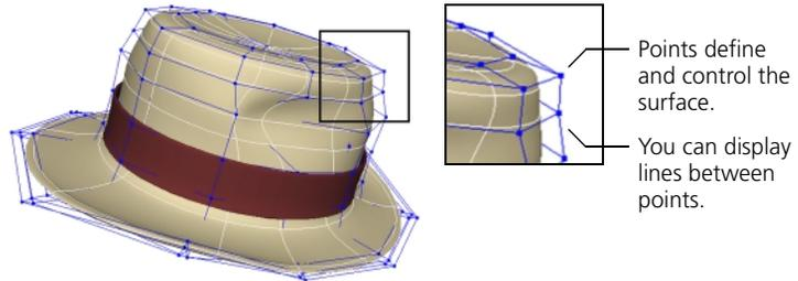
You cannot add or remove points directly, but you can add and remove knots as described in *Working with Knots and Knot Curves* on page 100—this has the effect of adding or removing points indirectly.
