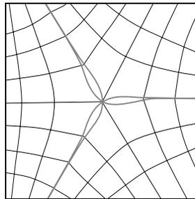
Simply joining them at the central point causes overlapping edges.
