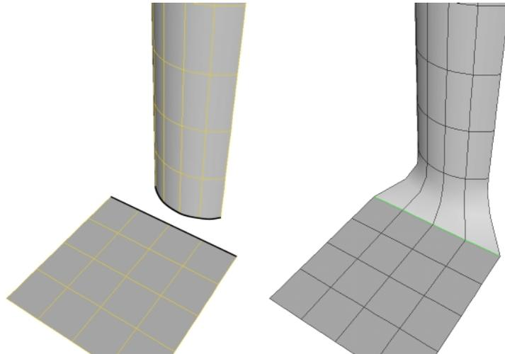
3. Assemble the surfaces into a single surface mesh.
